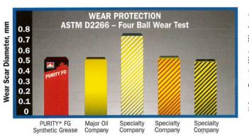
PURITY FG Synthetic delivers equal or better wear protection than the leading major oil company's and specialty lubricant suppliers' synthetic food grade greases. Less wear means fewer production upsets, higher productivity and lower maintenance costs.
