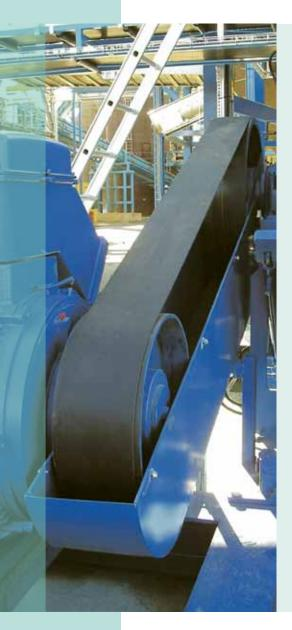
Siegling Extremultus belts excel at transmitting vast amounts of power proficiently. They are extremely efficient and often a welcome alternative to high-loss gear boxes.
