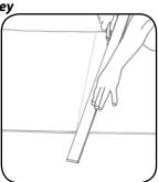
Measure the thickness of the carcass or the belt to choose the correct screw length and the right kind of Super-Screw<sup>®</sup>. For a better passage over the rollers and the scrapers, provide a bias installation. Cut your belt with a 1/3 bias (or 10% min of the width of the belt). The other side of the belt should be cut with a bias in the opposite direction.
