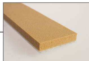
Sylomer, brown Polyurethane foam (bulk density: 400 kg/m 3 )
