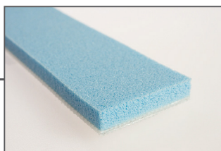
Sylomer, blue Polyurethane foam (bulk density: 220 kg/m 3 )
