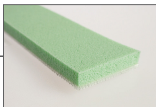
Sylomer, green Polyurethane foam (bulk density: 300 kg/m 3 )
