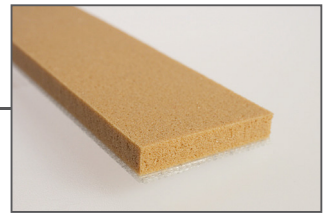
Sylomer, brown Polyurethane foam (bulk density: 400 kg/m 2 )
