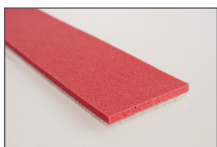
Sylomer, red Polyurethane foam (bulk density: 510 kg/m 3 )
