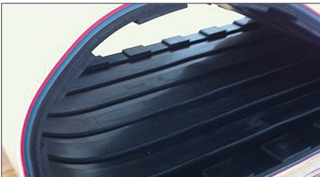
Conveyor belt for transporting rotor blades
