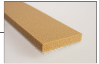
Sylomer, brown Polyurethane foam (bulk density: 400 kg/m 2 )
