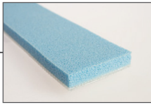
Sylomer, blue Polyurethane foam (bulk density: 220 kg/m 2 )
